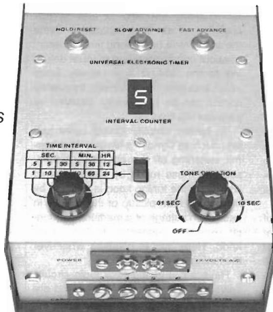
*Time any event occurring in a 24 hour period in seconds, minutes or hours. Includes audible alert and automatic on/off.*
